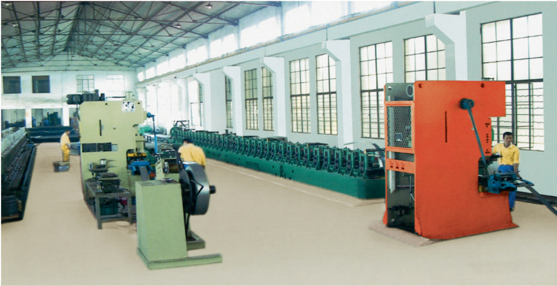
桥架自动成型生产线 automatic production line of cable tray
